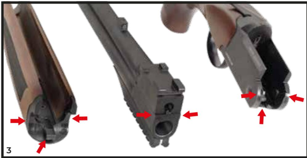
**3.** Attach barrels to the action by pushing the top lever to the right and engaging the dual hinge pin bearing notches on each side of the barrel. Hold the barrels with the muzzle at a downward angle with respect to the receiver. Once the bearings are properly seated, lift up on the barrels and close the action.
