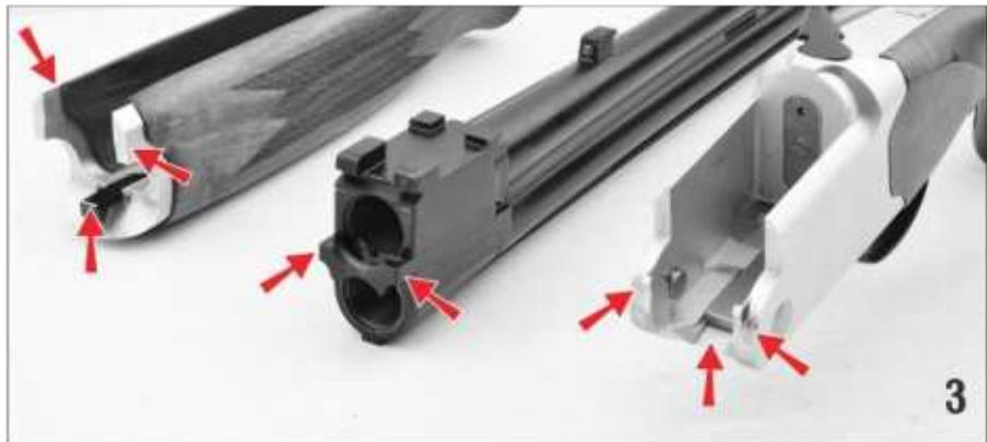
**3.** Attach barrels to the action by pushing the top lever to the right and engaging the dual hinge pin bearing notches on each side of the barrel. Hold the barrels with the muzzle at a downward angle with respect to the receiver. Once the bearings are properly seated, lift up on the barrels and close the action.
